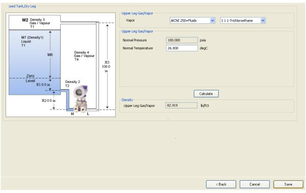
Figure 719. Sample IMV31 Transmitter Application Design Conditions - Closed Tank Dry Leg -Upper Leg Gas/Vapor - AlChE 250+ Fluids
