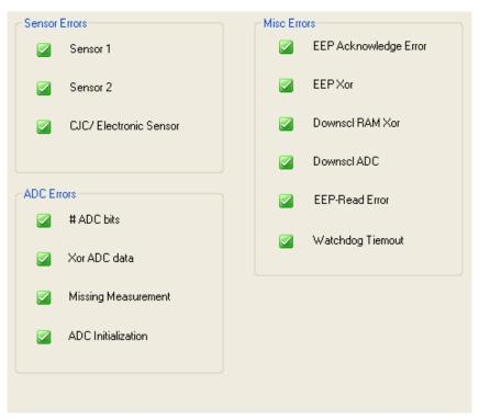
Figure 836. Sample RTT15 Transmitter Device Status Screen
