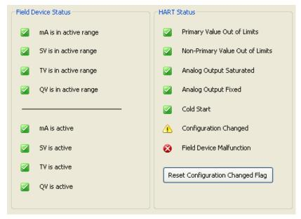
Figure 51. Sample CFT51 Transmitter HART Status Screen
