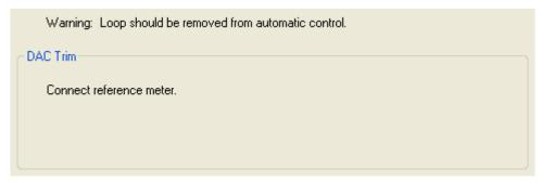
Figure 838. Sample RTT15 Transmitter DAC Trim Calibration Screen 1
