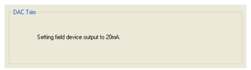
Figure 843. Sample RTT15 Transmitter DAC Trim Calibration Screen 6
