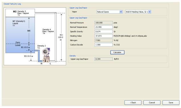
Figure 724. Sample IMV31 Transmitter Application Design Conditions - Closed Tank Dry Leg -Upper Leg Gas/Vapor - Natural Gases Screen (AGA-8 Heating Value Selection)
