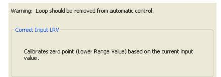
Figure 560. Sample I/A Series Advanced Pressure Transmitter Correct Input LRV Screen
