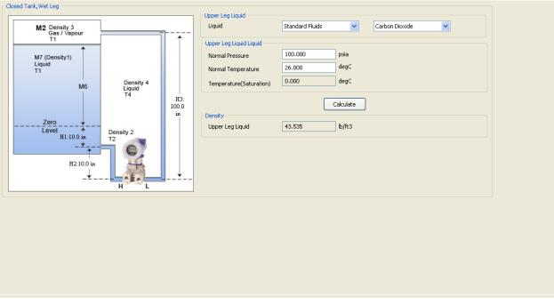
Figure 739. Sample IMV31 Transmitter Application Design Conditions - Closed Tank Wet Leg -Upper Leg Liquid - Standard Fluids
