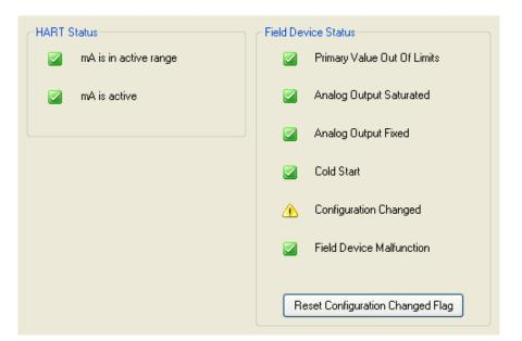
Figure 837. Sample RTT15 Transmitter HART Status Screen
