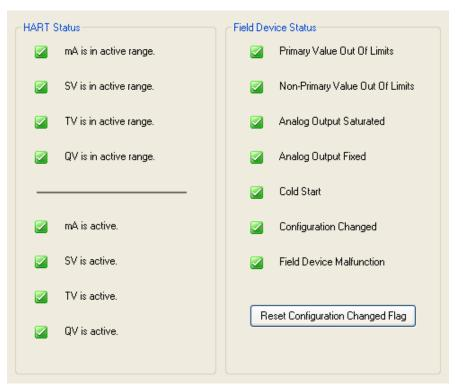
Figure 302. Sample 875EC Analyzer HART Status Screen
