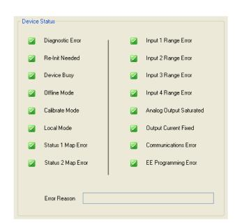
Figure 531. Sample I/A Series Pressure Transmitter Device Status Screen
