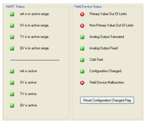
Figure 381. Sample 876EC Transmitter HART Status Screen
