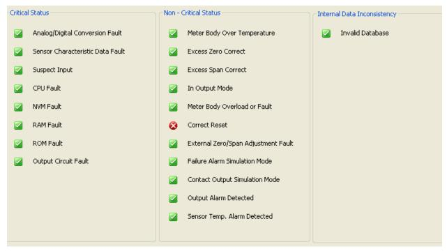
Figure 555. Sample I/A Series Advanced Pressure Transmitter Device Status Screen
