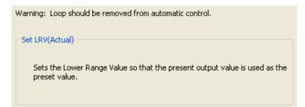
Figure 548. Sample I/A Series Advanced Pressure Transmitter Set LRV Screen
