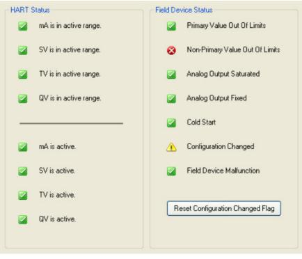
Figure 769. Sample IMV30 Transmitter HART Status Screen
