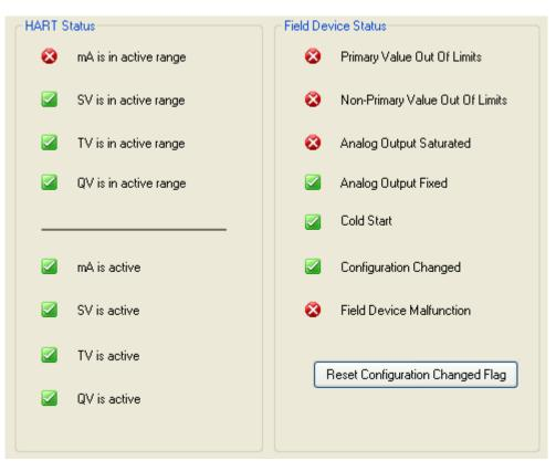
Figure 245. Sample 876PH Transmitter HART Status screen
